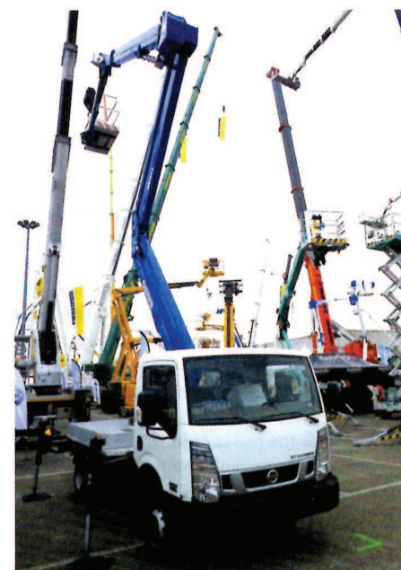
Isoli had a new truck mount on show, the 21m working height PNT210JD4
